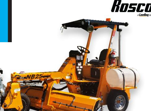
The NB25 is LeeBoy's 3 Wheeled Self-Propelled Sweeper. This broom is Designed with the Paving Professional in Mind® who is in need of a reliable and quality built 3 wheel sweeper. The frame is heavy duty, operator area is ergonomically friendly with optional climate controlled cab and the machine is easy to tow, if desired. The NB25 is perfect for the rental industry or general application sweeping for any surface with its heavy duty brush core.
