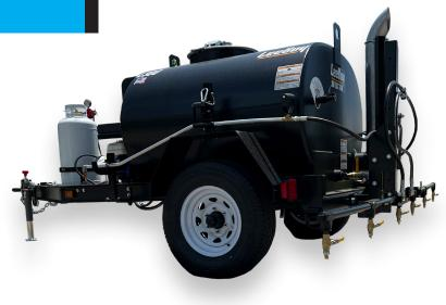
Perfect for the all-inclusive commercial paving contractor, the L300 Tack Distributor provides a perfectly sized tank for small to large projects including parking lots, patching, driveways or soil stabilization. Daily task can be completed with ease by relying on the trouble-free gas powered engine and the proven reliable user-friendly design. Uniquely configurable, the customizable options give the contractor the ability to create a solution specific to their exact needs.
