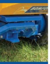
Rear protection Fitted with rear protection bar and towing anchor point.
