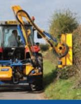
Hydraulic slew & breakout 110° of slew and hydraulic breakout makes the Osprey very adaptable.
