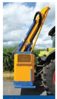
Slimline compact transport position Keeping weight closer to tractor for faster road speeds.
