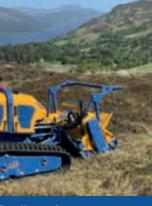
Excellent grip characteristics Individual tracks can be extended by up to 250mm (10").
