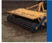
Crumbler roller Break down soil clods to give a fine finish ready for drilling.
