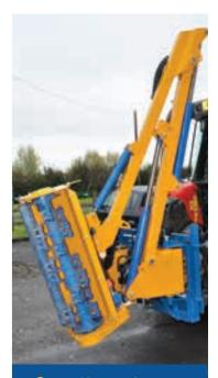
**Compact transport** As a result of the 110° power slew the Osprey has a compact inline transport position.
