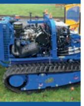
Perkins engine accessibility Removable steel engine panels for easy access.
