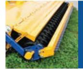
Packer roller Consolidate and break down soil to reduce soil
