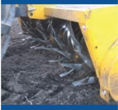
Front rotor Tines lift soil and turns into rear rotor to break down soil structure.
