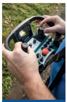
**Precise control** The remote control, operating all Flailbot functions has a range of 150m (492′).
