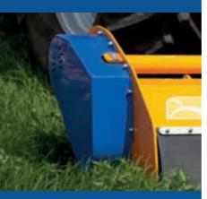
Easy adjustment Simple belt tensioning system with oil filled drive tube.
