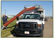
Hydraulically powered **Litter Loder** is a powerful vacuum and eliminates auxillary engine noise.
