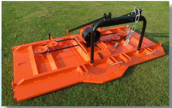
All generously overlapping cutting blades are driven indirectly by means of V-belts, mostly with automatic springloaded belt tensioners. This flexible drive system protects the gearbox from shock loads.
