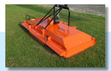
LF-type Rotary Mowers have long, rounded skids at both sides to allow for fast working speeds (up to 8-10 km/h = 6-6.5 mph).
