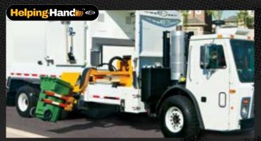
Collect from the comfort of the cab while still having the option to pick up extra items left on residential routes. The Helping-Hand™ arm has a pivot point that provides a minimal swing-out motion, making it ideal for dumping in narrow spaces and alleys. It can extend up to 10 feet and lift up to 400 pounds when fully extended. By being located inside the hopper, the Helping Hand eliminates the need to compensate for torsion stress, reducing wear and tear on the arm's components.
