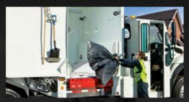
The Expert drop frame configuration is perfect for manual or semi-automated waste or recycling collection, and the loading height of only 5.5" above the chassis frame makes this configuration safer, faster, and easier to load. With the shortest wheelbase in the industry, this truck can easily maneuver in some of the tightest spots where other drop frame converters cannot.
