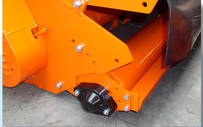
A full width rear roller and skids at both sides provides excellent stability and easy handling. To protect the bearings of the rear rollers, the bearings are fitted with unique covers to prevent humidity, dust and mud from entering.
