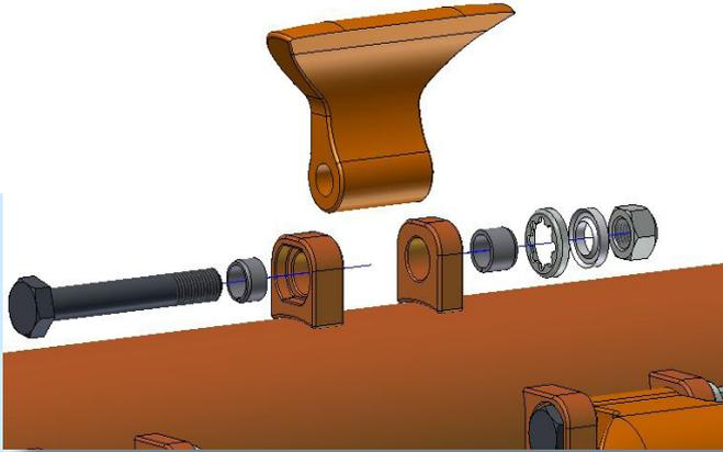
2,2 kg (5 lbs) heavy-duty "PERFECT" flails are especially designed for pulverizing prunings. They are fitted to the double electronically balanced flail rotor with heavy bolts and replaceable steel bushings. They provide an excellent pulverization. Combi-flail are optionally available.
