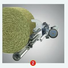
Once the net wrap has been picked up by the bale, the duckbill rotates back to the home position as net is dispensed into the chamber.
